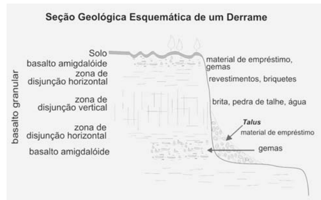
Figure 12 (below) - Schematic representation of the flow structures from Bacia do Paraná volcanism.
