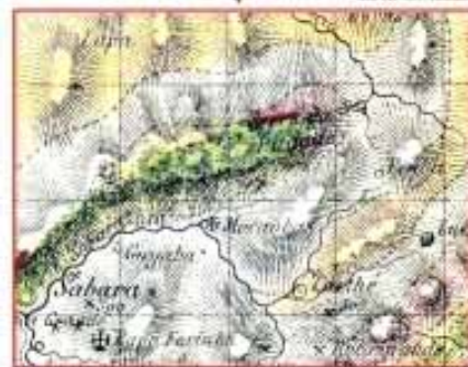
Figure 8 - Geological map of Quadrilátero Ferrífero by P. Claussen (1841), in detail the Serra da Piedade, green is the so-called “siderochriste” (iron formation).
